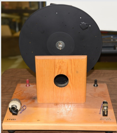
Don Menning's early mechanical television reproductions. Lots of woodworking skill and electronic engineering to reproduce what was invented in the early 1900s.
