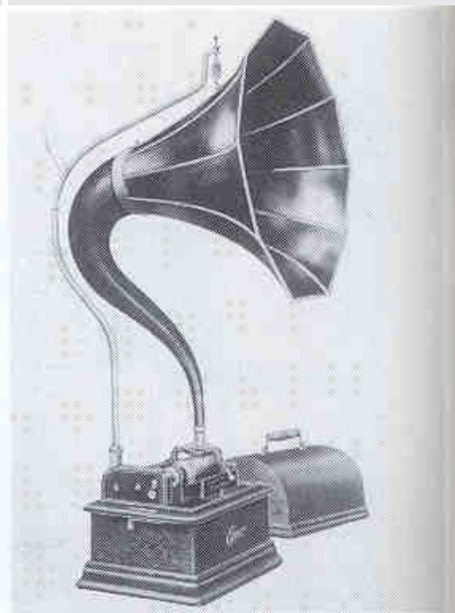
Edison "Standard" phonograph of 1911 with cygnet horn and supporting crane. Reproducer was Type O turnover. Played both two- and four-minute records. (Edison National Historic Site Museum.)
