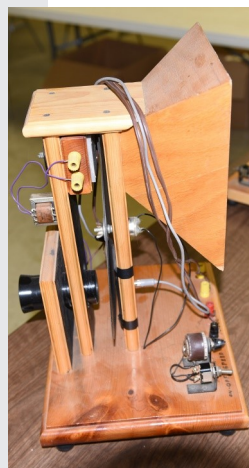
Don Menning's early mechanical television reproductions. Lots of woodworking skill and electronic engineering to reproduce what was invented in the early 1900s.
