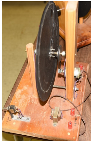
Don Menning's early mechanical television reproductions. Lots of woodworking skill and electronic engineering to reproduce what was invented in the early 1900s.
