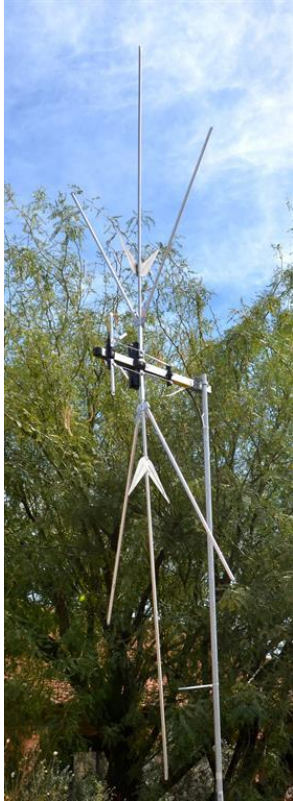
Fig. 3: A quality antenna is essential to ensure a receiver that works well. Shown is the SCANNER ANT-BASE model antenna from AntennaCraft, which works from 30 to 1300 MHz. (Click to Enlarge)
