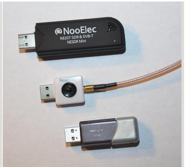
Fig. 2: Shown top to bottom, the Realtek 2832RTL-based receiver in a USB package, a nano USB receiver with RF adapter cable and a standard small USB memory stick. (Click to Enlarge)
